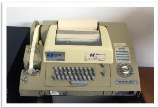
A Telex machine with ticker tape to send and receive telegrams
