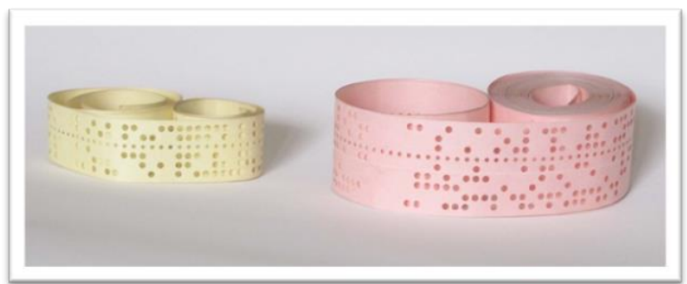
Computer punched tapes, 5- and 8-hole.
