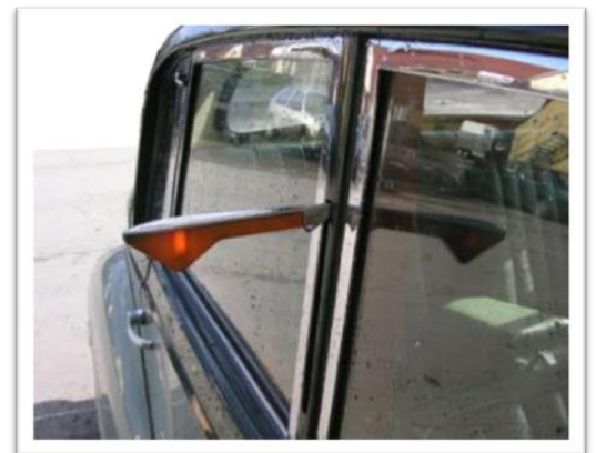
Electro-mechanical indicator or trafficator
