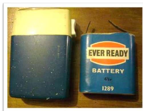
Torch or Flashlight with 4.5 volt battery
