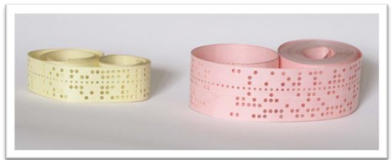
Computer punched tapes, 5- and 8-hole.
