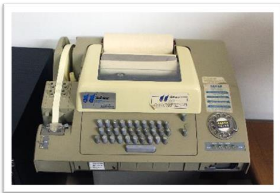
A Telex machine with ticker tape to send and receive telegrams
