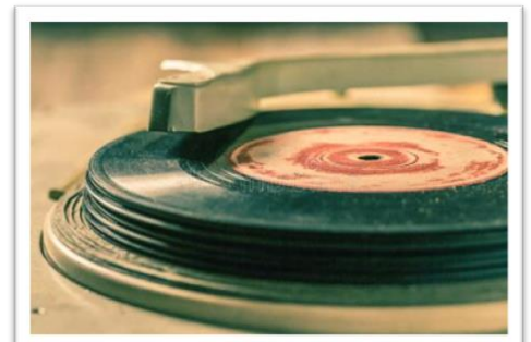
A record player with a stack of "45's" or 'singles'. Earlier records were 78 rpm, and later LP's were 33\frac{1}{3} rpm.
